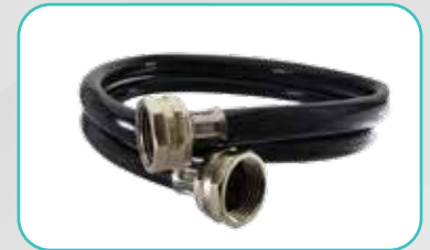
CONECTOR P/LAVADORA 3/4" X 3/4" X 120 CM TEMPERATURA 0°C - 60°C PRESION 7KG/CM2
